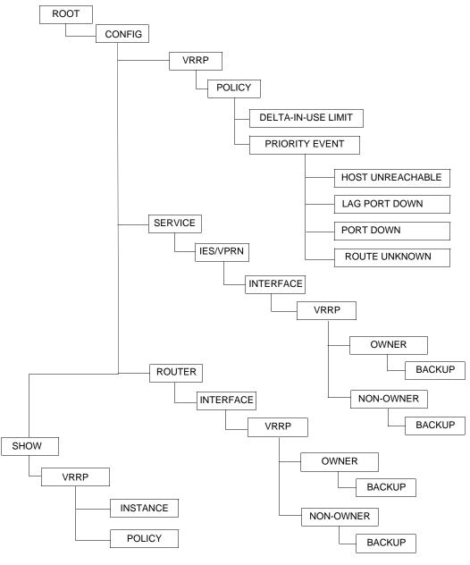
Figure 18: VRRP Command Structure
